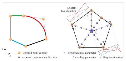
Figure 1 Scaled-Boundary Isogeometric Analysis Parameterization
